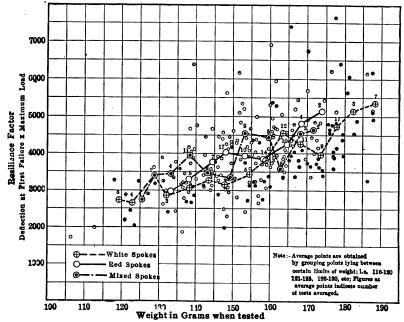
Fig. 53.—Spoke-test chart, showing relation between resilience factor and weight in clear spokes.
